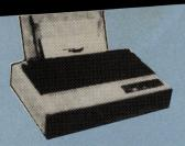
Hugely successful 9 pin printer, the Star LC10 provides 4 NLQ fonts (with 96 print combinations) at 36cps and 144cps draft. Has a large 4K buffer and IBM/parallel interface built in, includes a comprehensive front panel operation and features paper parking, allowing single sheets to be used without removing tractor paper.
